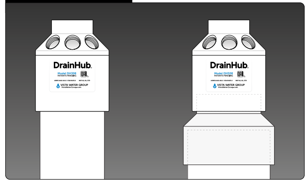
3" Pipe into Hub
